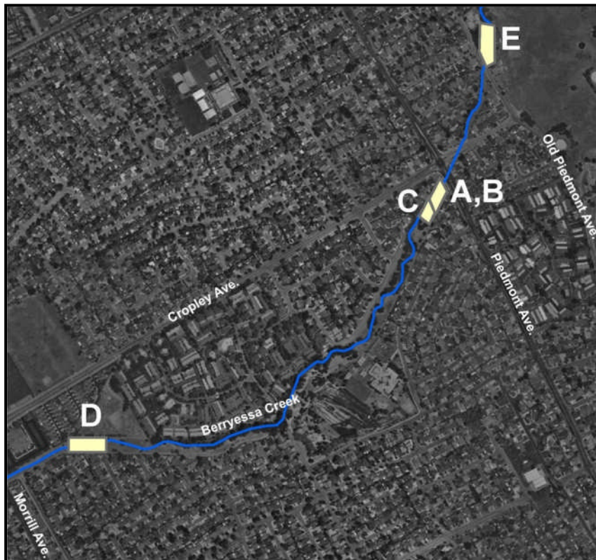
Figure 3-13 Plan View of Alternative Sediment Basin Configurations
