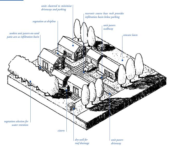
**7.1c High density multi-family site.** In the Bay Area, many of the sites for new construction are infill or redevelopment sites. These sites usually have higher densities (typically from 12 to 40 units per acre) which demands a greater proportion of pavement and roof coverage.
