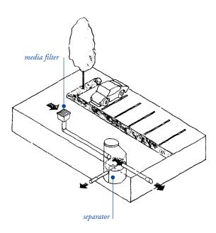
**S**ome areas are so densely developed that streets, buildings and walkways provide almost complete impervious land coverage. Here, land values prohibit the use of landscape solutions such as biofilters, infiltration basins, or wet ponds. In addition, the soil conditions in these highly urbanized locations often do not support infiltration, further reducing the practicality of landscape stormwater quality systems.
