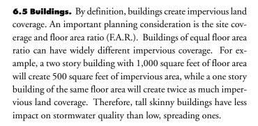
Once the building size and coverage is determined, there are a limited number of techniques for managing runoff from individual buildings to collect rooftop runoff and allow it to infiltrate into the soil.
