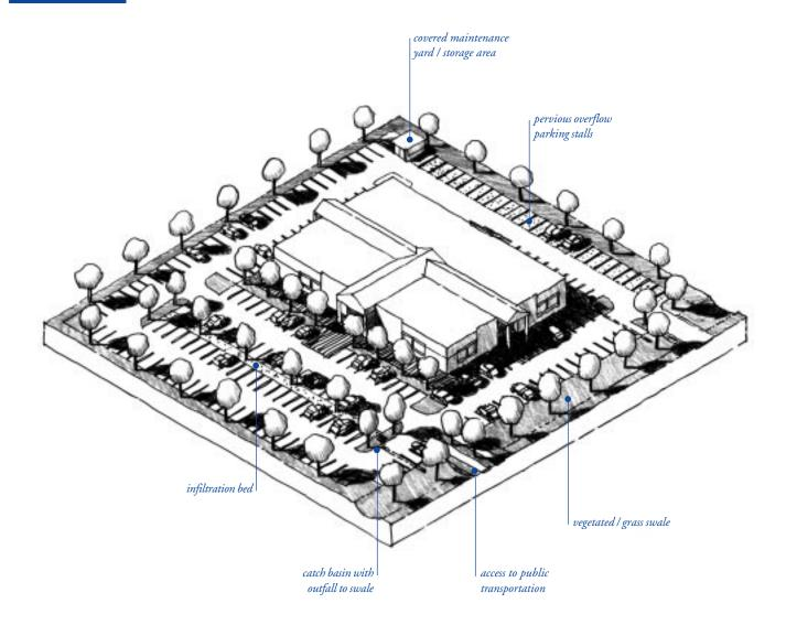
**7.2a Shopping center.** Shopping centers present many opportunities for stormwater management, especially in the parking areas. Infiltration swales and extended detention (dry) basins can be incorporated into space between parking aisles. Recognizing that much of the parking is only necessary during peak times, such as the holiday season, a proportion of outlying stalls may be paved with a more permeable pavement such as crushed aggregate or turfblock.
