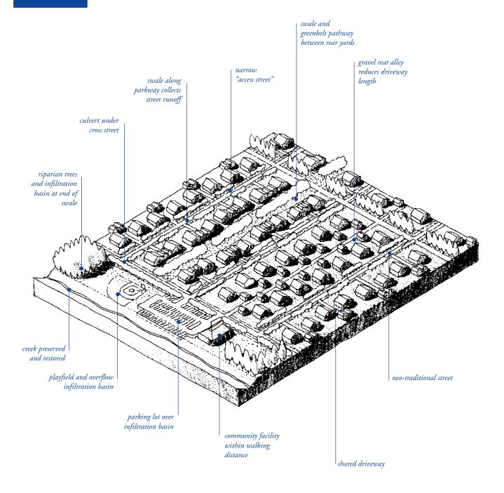
**7.1f Large flat site.** Larger flat sites present some of the greatest opportunities for stormwater management. If soils have adequate percolation rates, infiltration swales and basins are easily incorporated. In more poorly drained soils, flat sites allow for detention and retention systems to slow the speed of runoff and hold it for later release. This allows sediments to settle and minimzes stream bank erosion from high velocity flows.
