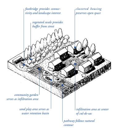
Unlike conveyance storm drain systems that hide water beneath the surface and work independently of surface topography, a drainage system for stormwater infiltration can work with natural land forms and land uses to become a major design element of a site plan.
