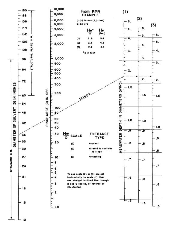
Figure CU-26—Headwater Depth for Corrugated Metal Pipe Culverts With Inlet Control
