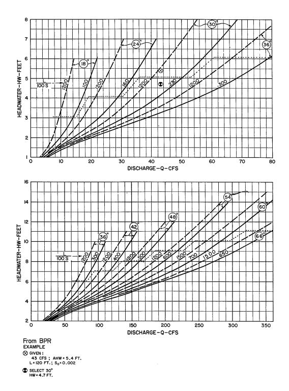
Figure CU-7—Culvert Capacity Chart—Example
