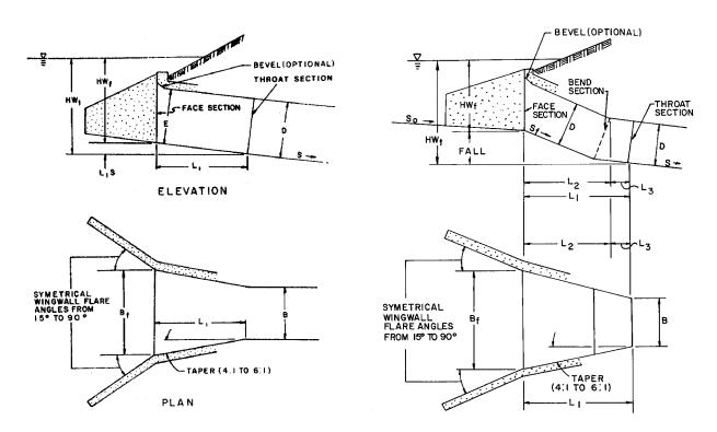
Figure CU-14—Side-Tapered and Slope-Tapered Improved Inlets
