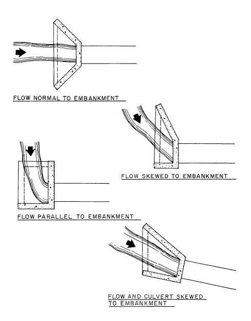
Figure CU-13—Typical Headwall-Wingwall Configurations
