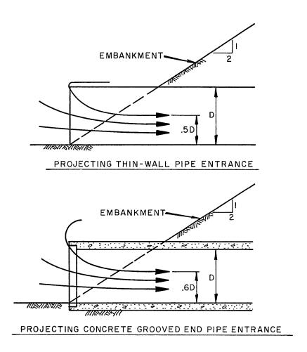
Figure CU-11—Common Projecting Culvert Inlets
