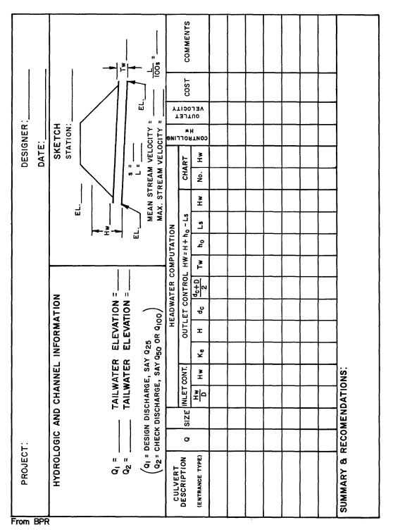
Figure CU-8—Design Computation for Culverts—Blank Form
