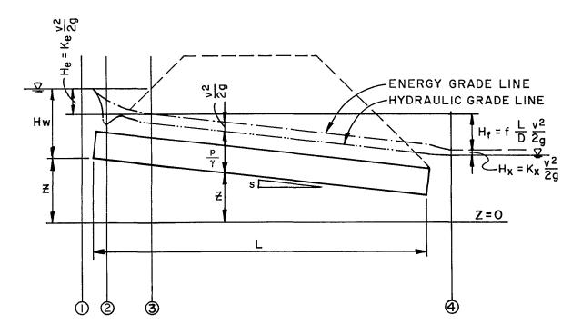
Figure CU-1—Definition of Terms for Closed Conduit Flow
