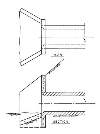
Figure CU-12—Inlet With Headwall and Wingwalls
