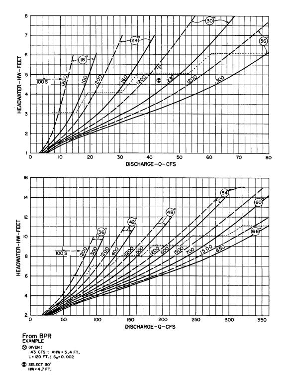
Figure CU-24—Culvert Capacity Circular Concrete Pipe Groove-Edged Entrance 18" to 66"
