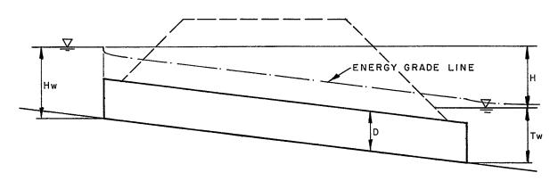
Figure CU-6—Outlet Control—Full Conduit
