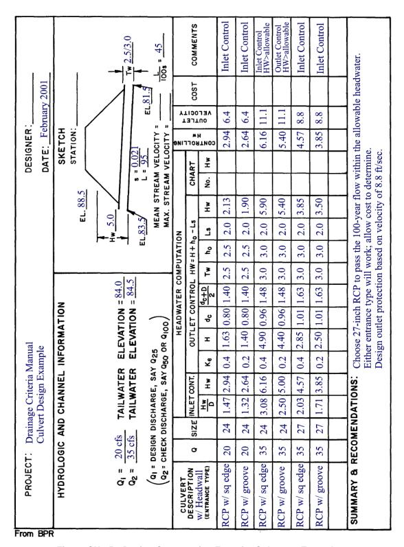
Figure CU-15—Design Computation Form for Culverts—Example 9.1
