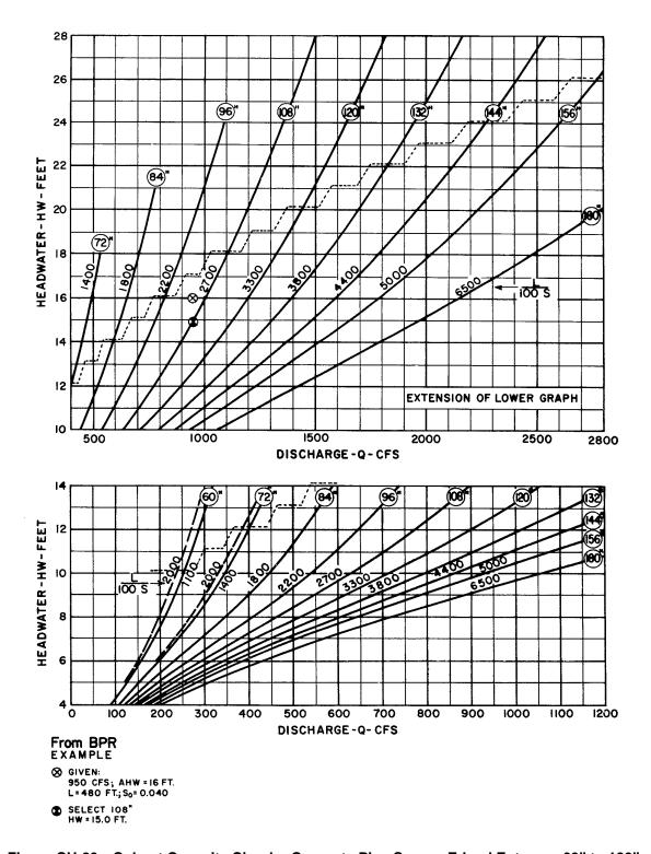
Figure CU-23—Culvert Capacity Circular Concrete Pipe Square-Edged Entrance 60" to 180"
