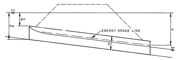
Figure CU-4—Inlet Control—Submerged Inlet
