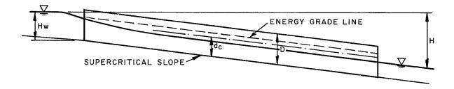
Figure CU-3—Inlet Control—Unsubmerged Inlet
