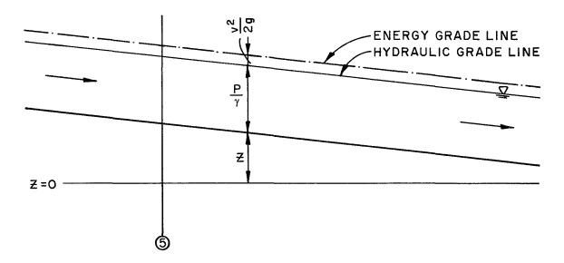
Figure CU-2—Definition of Terms for Open Channel Flow
