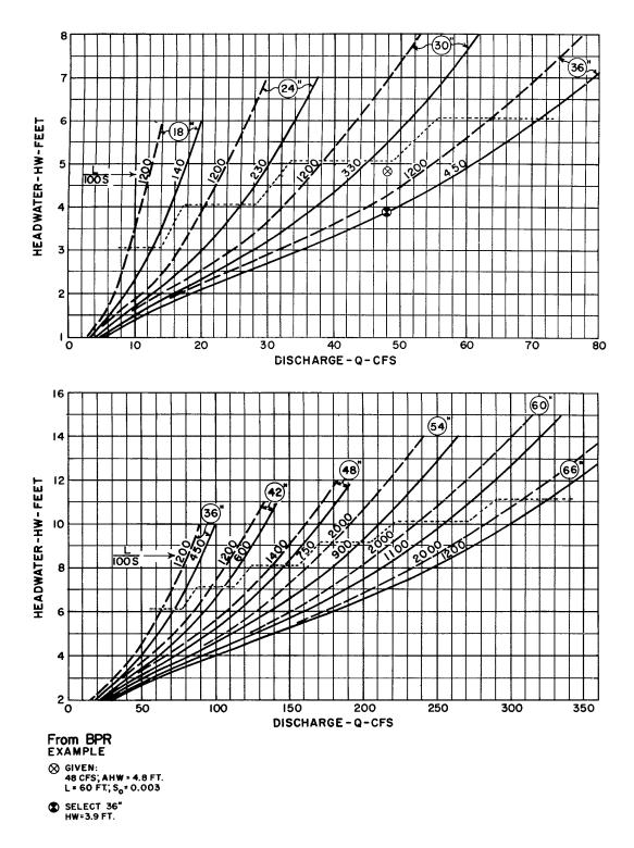
Figure CU-22—Culvert Capacity Circular Concrete Pipe Square-Edged Entrance 18" to 66"
