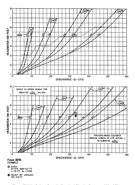
Figure CU-20—Culvert Capacity Standard Circular Corrugated Metal Pipe
