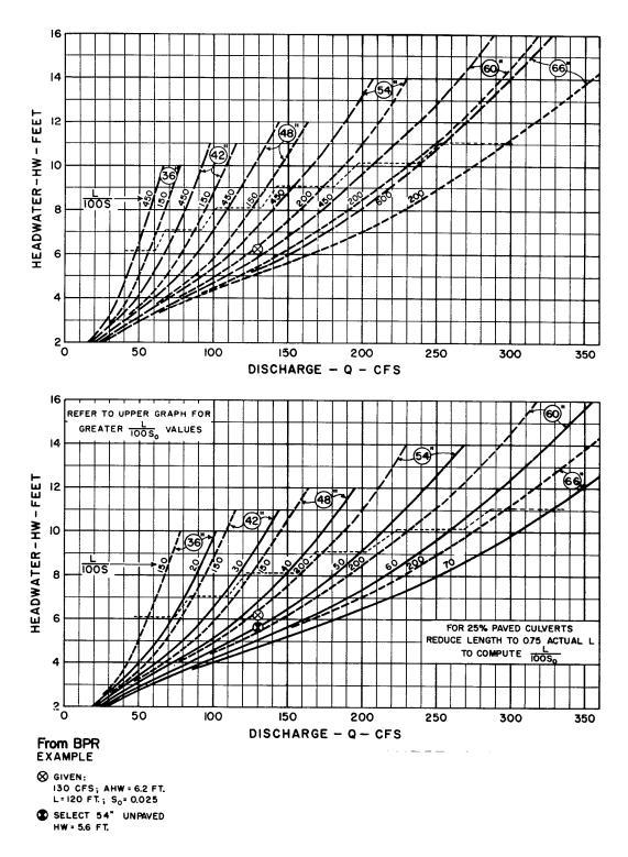
Figure CU-19—Culvert Capacity Standard Circular Corrugated Metal Pipe Headwall Entrance 36" to 66"
