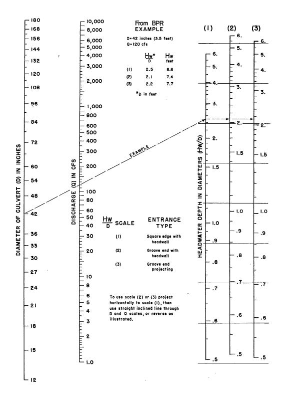
Figure CU-9—Inlet Control Nomograph—Example
