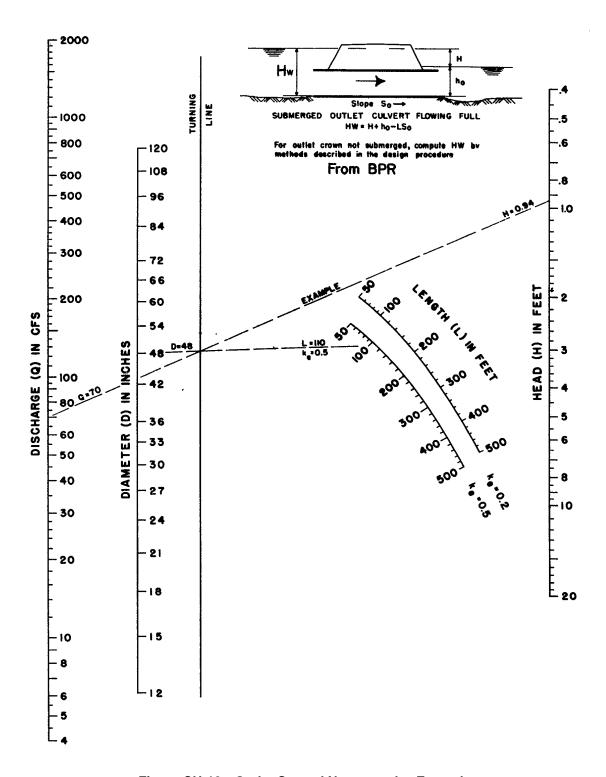
Figure CU-10—Outlet Control Nomograph—Example
