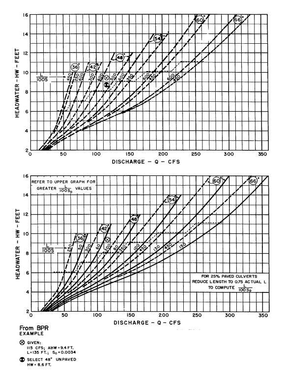
Figure CU-21—Culvert Capacity Standard Circular Corrugated Metal
