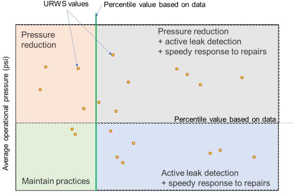
Real loss volumetric performance indicator e.g. Real loss per connection per mile per day
