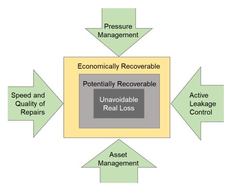
Figure 2 Foundational Approaches to Leak Detection
