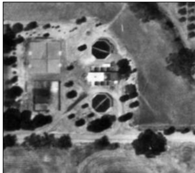
Figure 6: A 1948 aerial photograph (left) shows the treatment plant several years after completion. The sludge drying beds are on the left with the biofiltration system (trickling filters) and sludge digester structure at right. Note that the filters have two spraying arms versus the four now used. A 1965 photograph (right) shows that an addition had been constructed on the control room, visible at the right side of the sludge digester. 19
