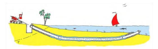
The system, called Neodren<sup>®</sup> provides extremely low turbid water as source water. Noncorrosive HDPE pipes with microporous sections (60  $\mu$ m or 120  $\mu$ m pores) are inserted 10 feet to 20 feet below the seafloor. The HDD laterals yield 1 to 2 MGD per lateral of source water without fish larvae, red tide algal and have no contribution or exacerbation of the seawater intruding into on the inland aquifer.
