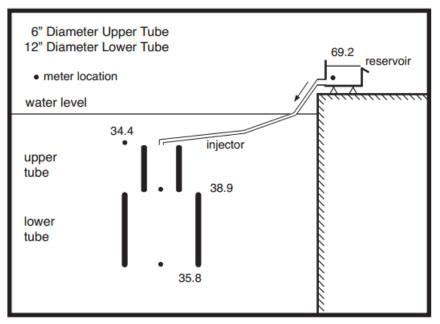
Salinity of the Effluent approximately 4% above the Ambient.
