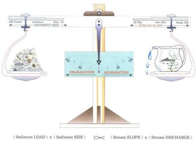
Figure 1 - Schematic of the Lane Relationship
