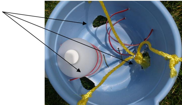
3. Place several well placed sample container straps within the bucket
