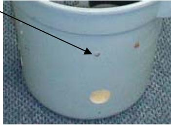
4. Attach a weight to the bottom of bucket. This example uses a dive weight being attached with two methods, cable ties and wire.
