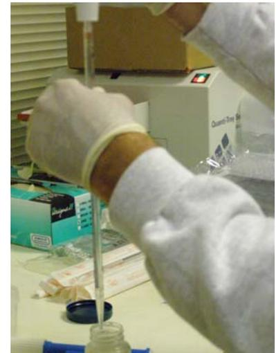
Prepare a sterile pipette and take some of the sample water (10ml or 1ml depending on Dilution rate desired).
