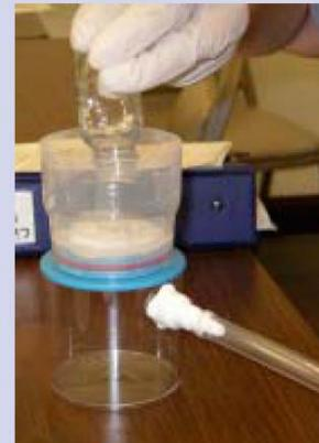
The water sample is filtered, then the filter is placed on Coliscan medium.
