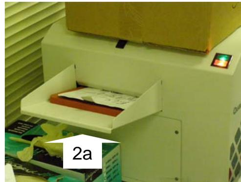
**3** Remove Quanti-Tray and insert. If they were inserted crooked you may stop and reverse the insertion and re-insert them.
