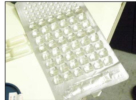
**4** Sealed Quanti-Tray removed from the rubber insert.
