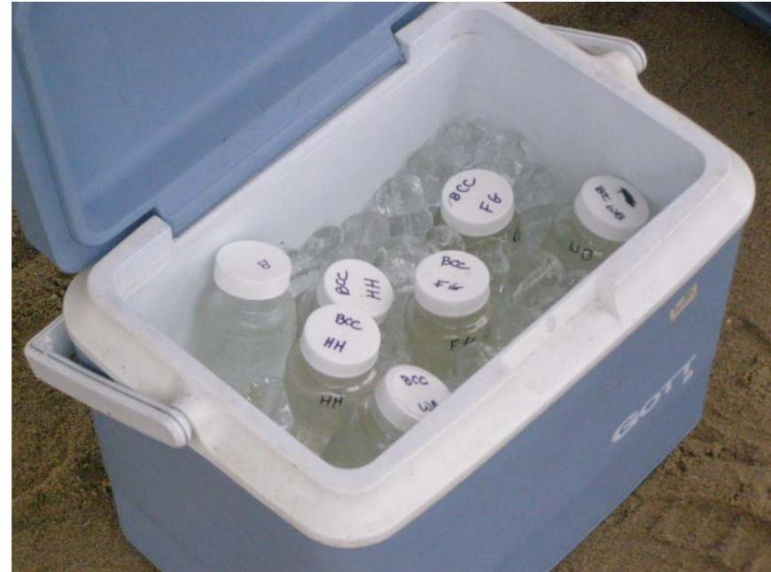
A **temperature blank** is a container containing only water. It is placed into the ice chest at the same time as the first water sample. When the samples are released to the lab, they will check the temperature of the temperature blank as a surrogate for a water sample
