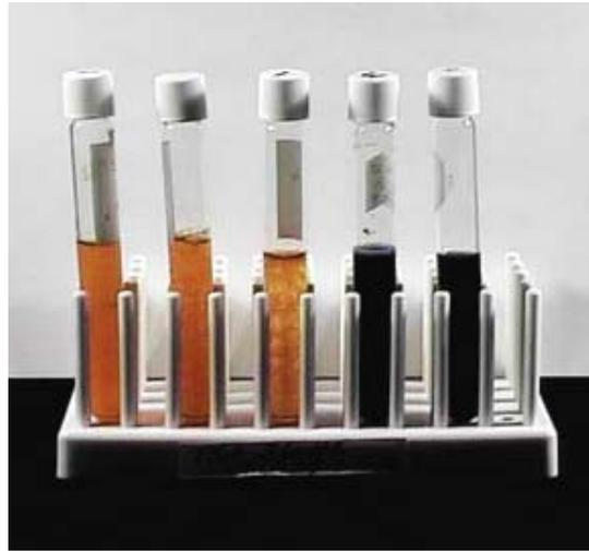
The **multiple-tube fermentation** method involves adding specified quantities of the sample to tubes containing a nutrient broth, incubating the tubes at a specified temperature for a specified time period, and then looking for the development of gas and/or turbidity that the bacteria produce. The presence or absence of gas in each tube is used to calculate an index known as the **Most Probable Number (MPN)**.
