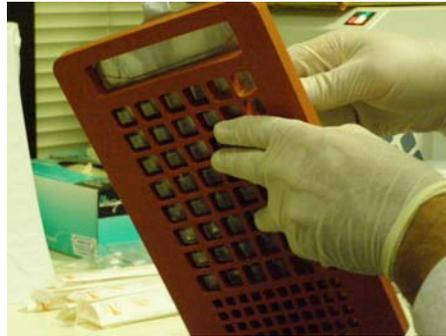
**2** Place the Quanti-Tray/Inset onto the input shelf and feed it into the sealer.
