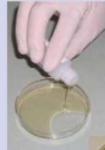
Water sample mixed with liquid Coliscan medium is poured into the Coliscan plate, which is coated with ingredients that cause the mixture to gel.
