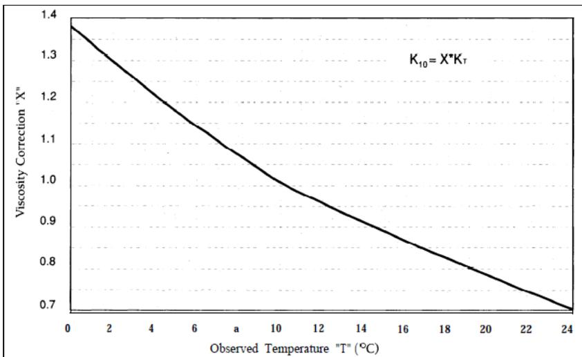
Figure 3. Permeability correction curve to account for viscosity changes with temperature
