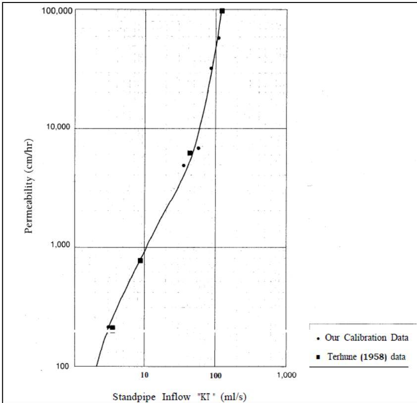
Figure 2. Permeability vs. standpipe inflow rate calibration curve.
