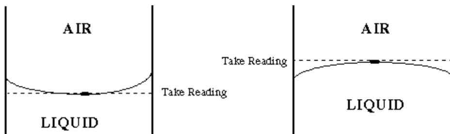
2. Record the reading, including units (inches), before removing the gauge from its base. After recording the value, double check your reading, then empty the gauge and reset it.
