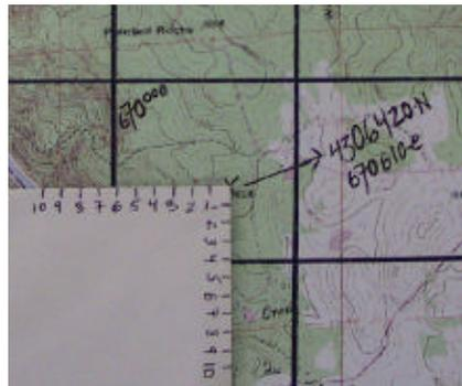
In the above example, the full easting coordinate value = 670000m.E, and the full northing coordinate = 4306000m.N. The ruler indicates that the 670000m.E. grid line intersects the horizontal scale at 61, making the easting coordinate 670610m.E. The 4306000m.N grid line crosses the vertical scale at 420 resulting in a northing coordinate of 4306420m.N.
