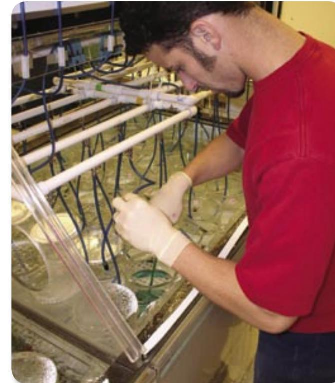
UCD staff captures fish exposed to surface water samples for analysis of EEDC activity.
