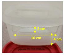
Figure 1. Ramp trap design.
