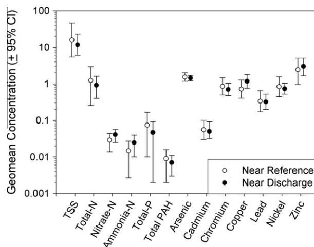
Fig. 2. Comparison of geometric mean (+95% confidence interval) concentrations in ambient near-shore receiving waters following storm events at reference drainage and ASBS discharge sites. Total suspended solids (TSS) and nutrients in mg/L; total polycyclic aromatic hydrocarbons (Total PAHs), and total trace metals in  $\mu\text{g/L}$ .
