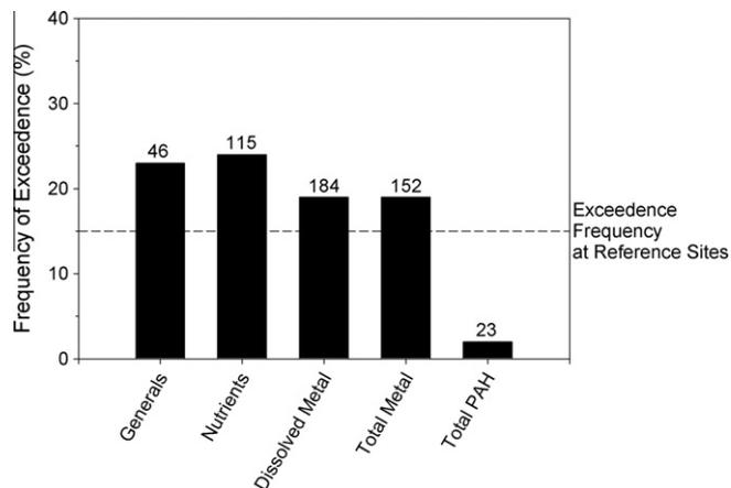
**Fig. 5.** Frequency of reference site based threshold exceedences by parameter group for all storm events and all Areas of Special Biological Significance (ASBS) in Southern California. Number above bar is total sample size.
