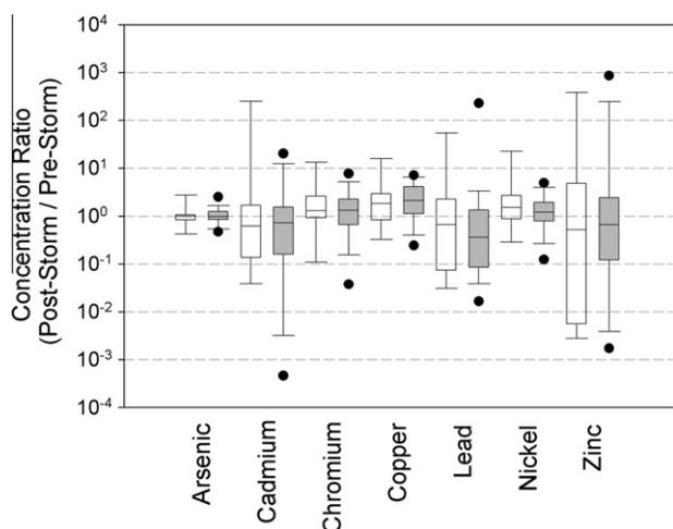
**Fig. 3.** Distribution of post-storm relative to pre-storm trace metal concentrations in ambient near-coastal waters at reference drainage (in white) and ASBS discharge (in grey) sites. Box plots include the 5th, 25th, 50th, 75th, and 95th percentile of the data distribution.
