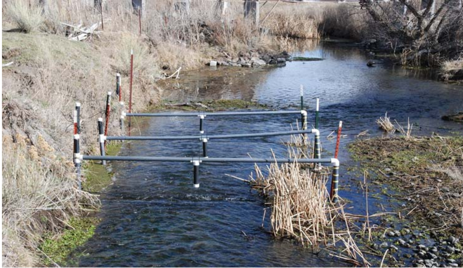
Photo 18. Directional Antenna System at HIG 1
