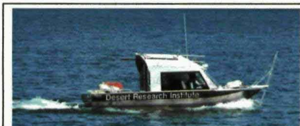
Fig. 6 The Desert Research Institute used a boat to measure the water quality near the shore of Lake Tahoe. The boat and water quality instruments inside can operate in poor and cold weather. The boat can also operate in very shallow water because it is equipped with a jet drive instead of a propeller. A probe on the bow was used to collect water samples while the boat was moving.
