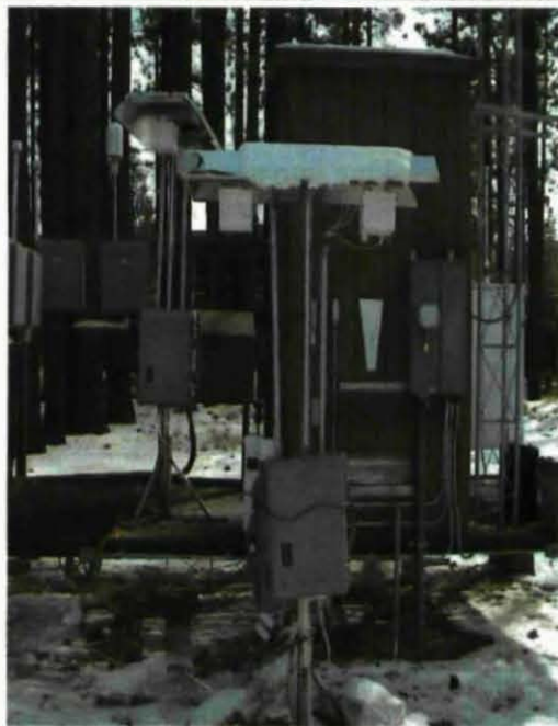
Figure 3. The Two Week Sampler (TWS) is the cornerstone of the LTADS monitoring program for nitrogen and phosphorus compounds that deposit to the Lake and contribute to algal growth. TWS measurements represent ambient conditions during every minute of the more than 1-year field study portion of LTADS.
