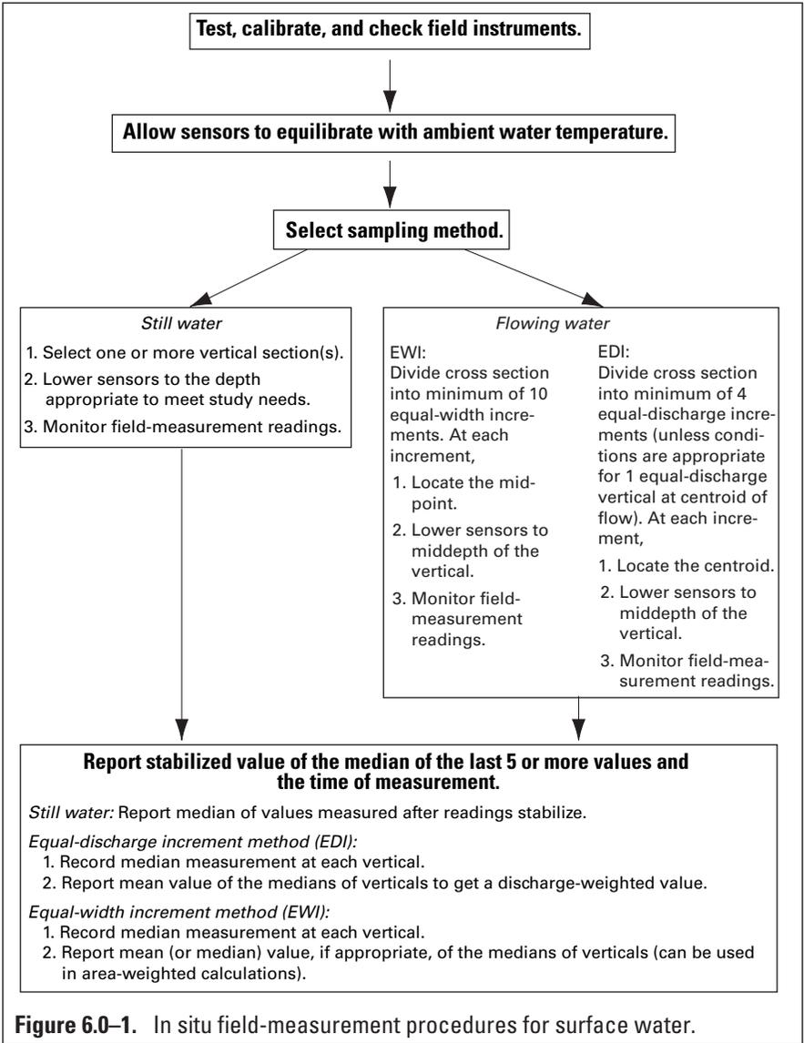
**Figure 6.0–1.** In situ field-measurement procedures for surface water.
