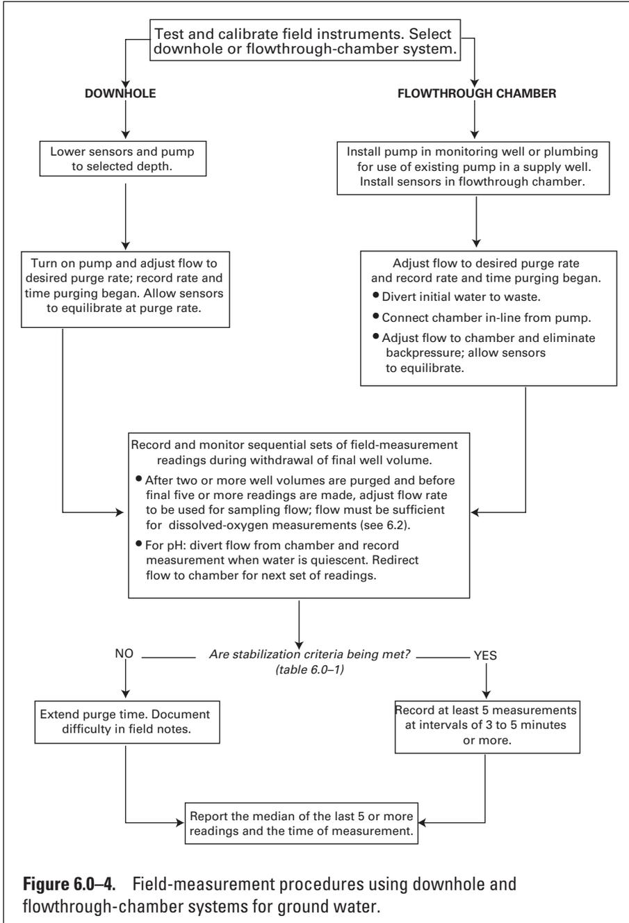
**Figure 6.0-4.** Field-measurement procedures using downhole and flowthrough-chamber systems for ground water.
