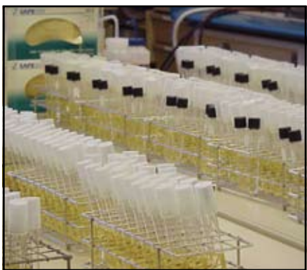
Multiple-Tube Fermentation Set-Ups
