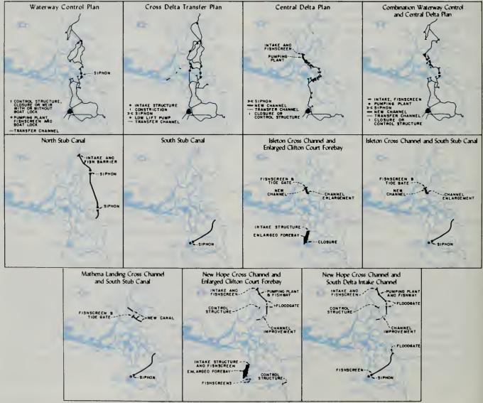
Figure B-10. Modified channel conveyance alternatives.
