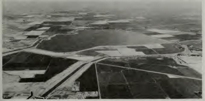
Clifton Court Forebay (center), which presently serves as the main diversion point for the SWP, will be terminus ad guem of the Peripheral Canal. As such, water regulated here will serve both the SWP Delta Pumping Plant (intake to the California Aqueduct, center left), and the CVP Tracy Pumping Plant, left loreground.
