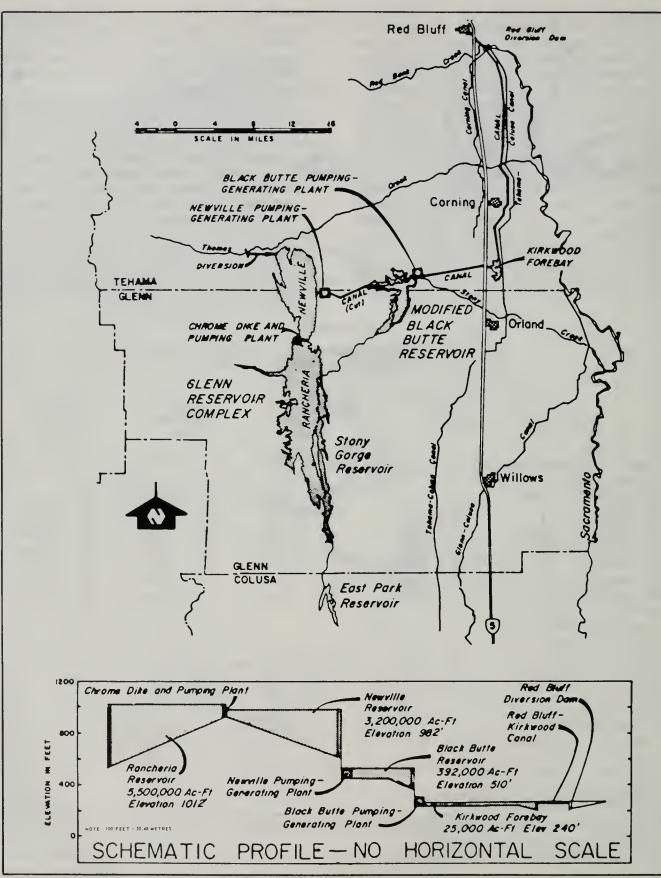
Figure 38. Glenn Reservoir - River Diversion Plan.
