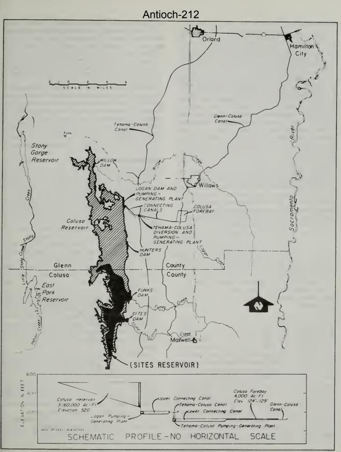
Figure 39. Colusa Reservoir - River Diversion Plan.
