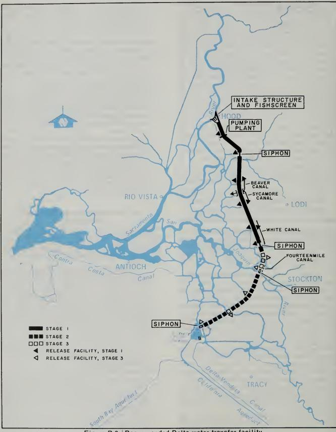
Figure B-8. Recommended Delta water transfer facility.
