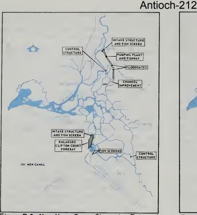
Figure B-2. New Hope Cross Channel – Enlarged Clifton Court Forebay Plan.
