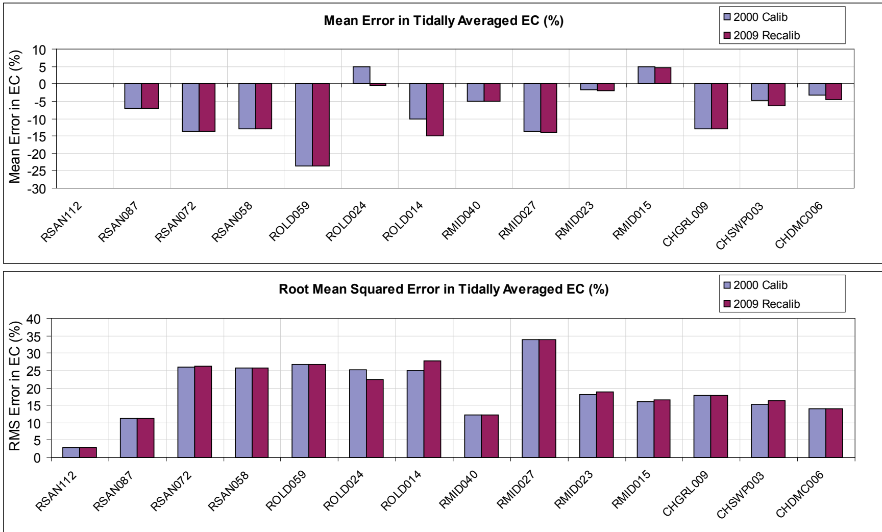
FIGURE 6-15 Summary of EC Calibration Metrics for Locations in the South Delta Region
