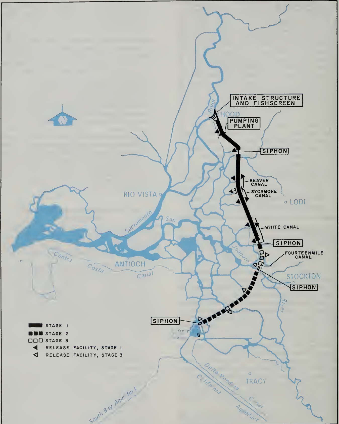
Figure B-8. Recommended Delta water transfer facility.
