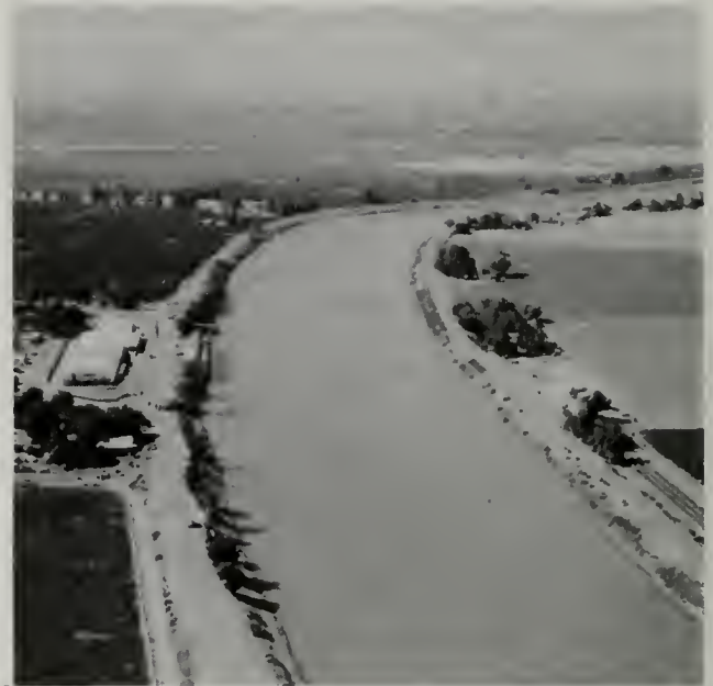
The Sacramento River at Hood, looking south. The Peripheral Canal would begin here, on the outside curve of the river, and run 42 miles south around the east side of the Delta to Clifton Court Forebay.
