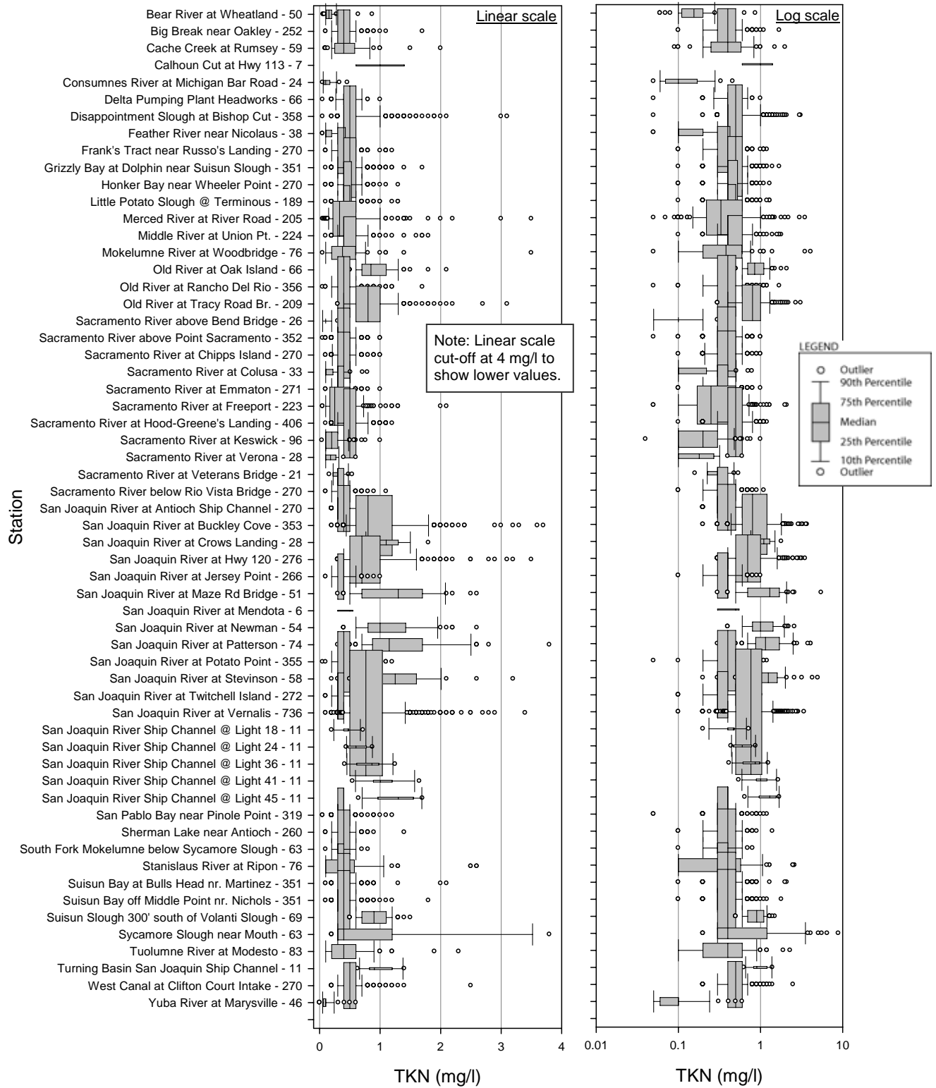
Figure 3-11. The range of TKN concentrations observed at different stations in the Central Valley and Delta. Box widths are proportional to the number of data points, shown next to station name.
