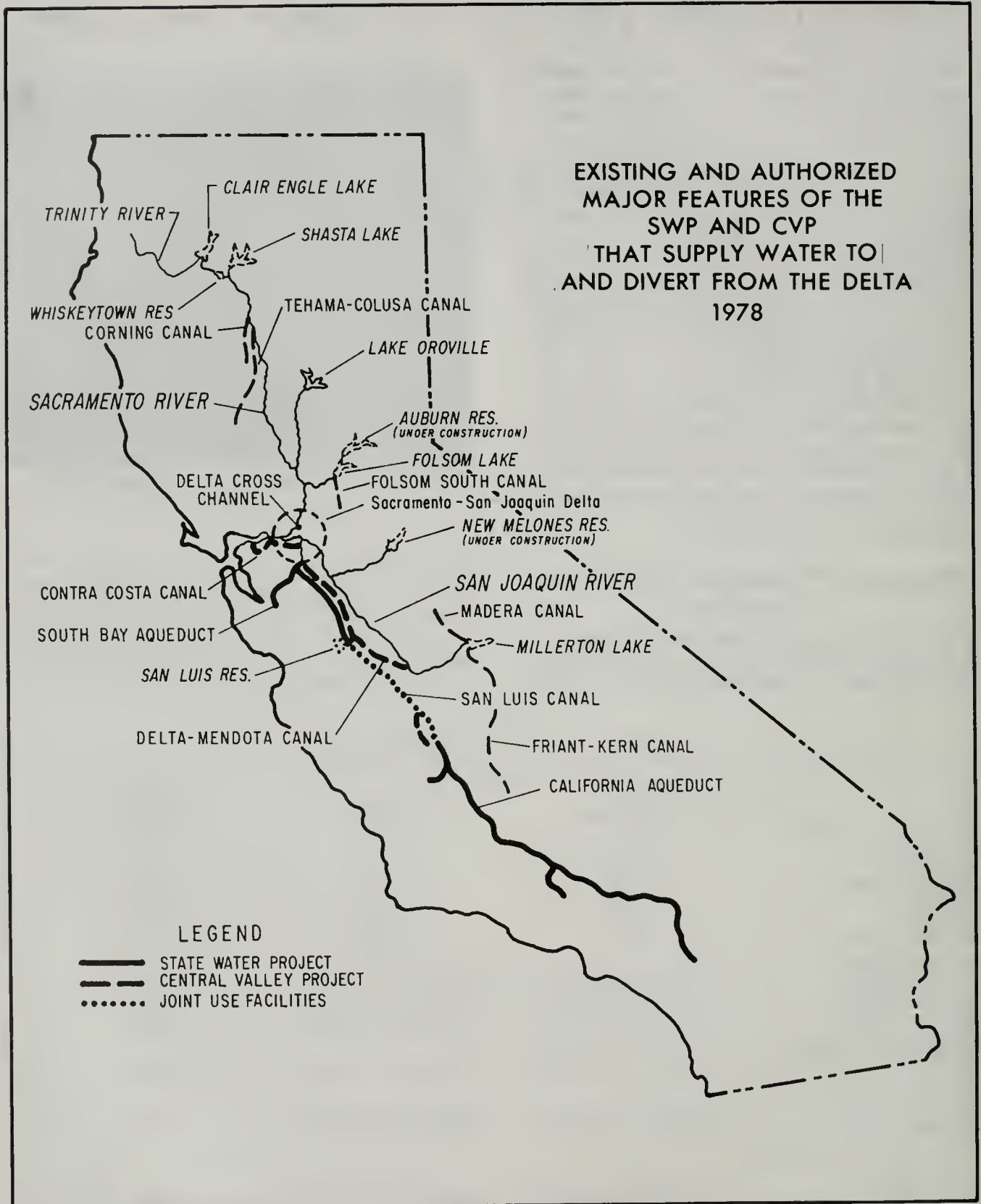
Figure 18. Major features of the SWP and CVP that supply water to and divert from the Delta, 1978.
