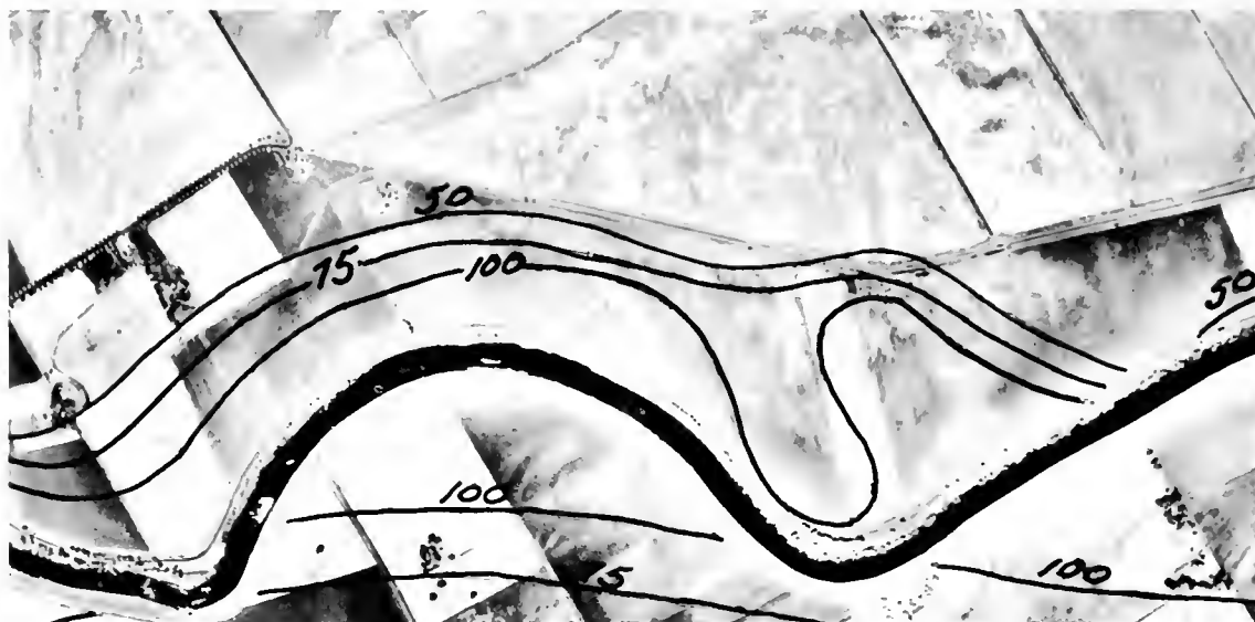
Figure 16. Lines of Equal Electrical Resistivity Near Miller's Landing
