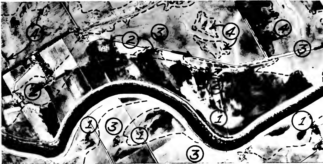
Figure 15. Identification of Seepage areas with Aerial Photography, Miller's Landing.
