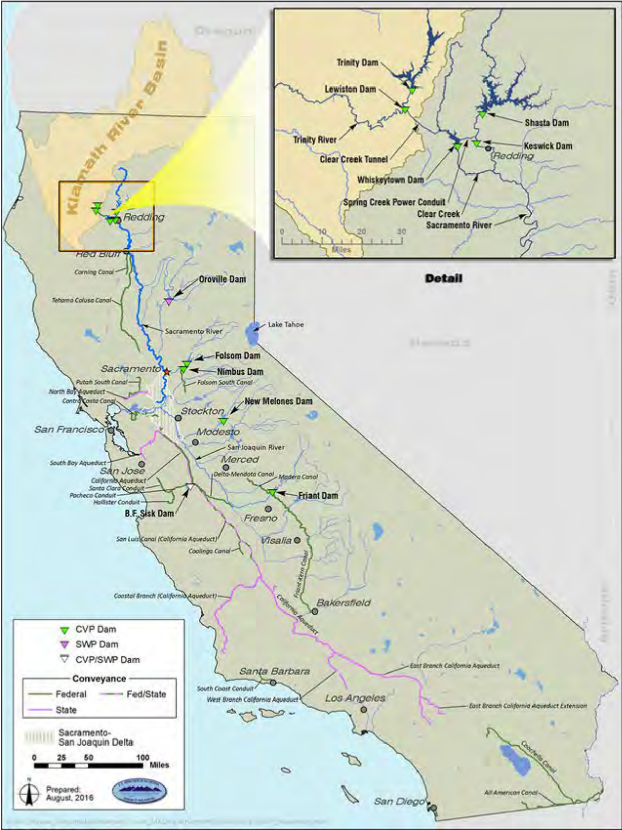
1 2 Figure 4-8. Major CVP and SWP Reservoirs, Downstream Rivers, and Conveyance Facilities
