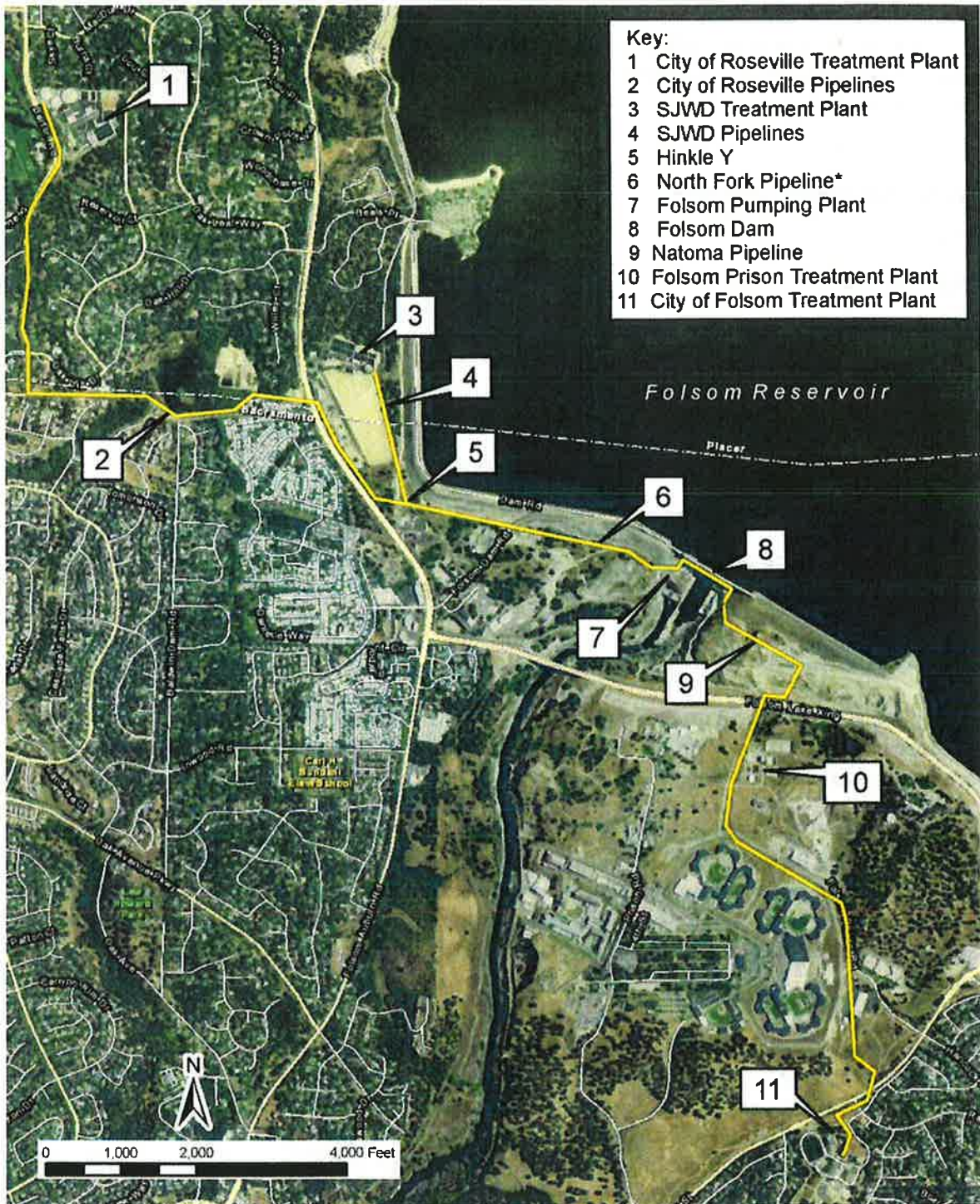
Figure 2-1 Raw Water Delivery System Layout
