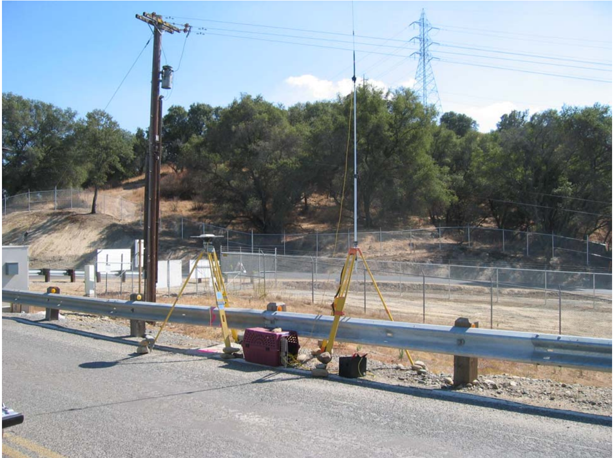
Figure 2- RTK GPS base station, WD48.
