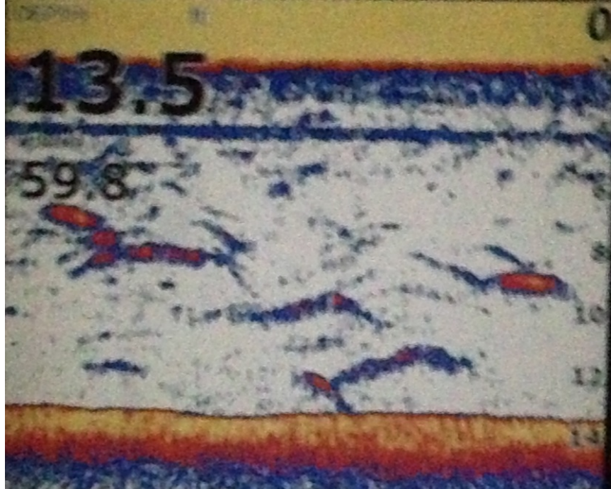
Figure 16. Depth sounder (“fish finder”) image of numerous large striped bass swimming in front of a large Sacramento River fish screen. Species determined by hook and line angling. Photo by Dave Jacobs.
