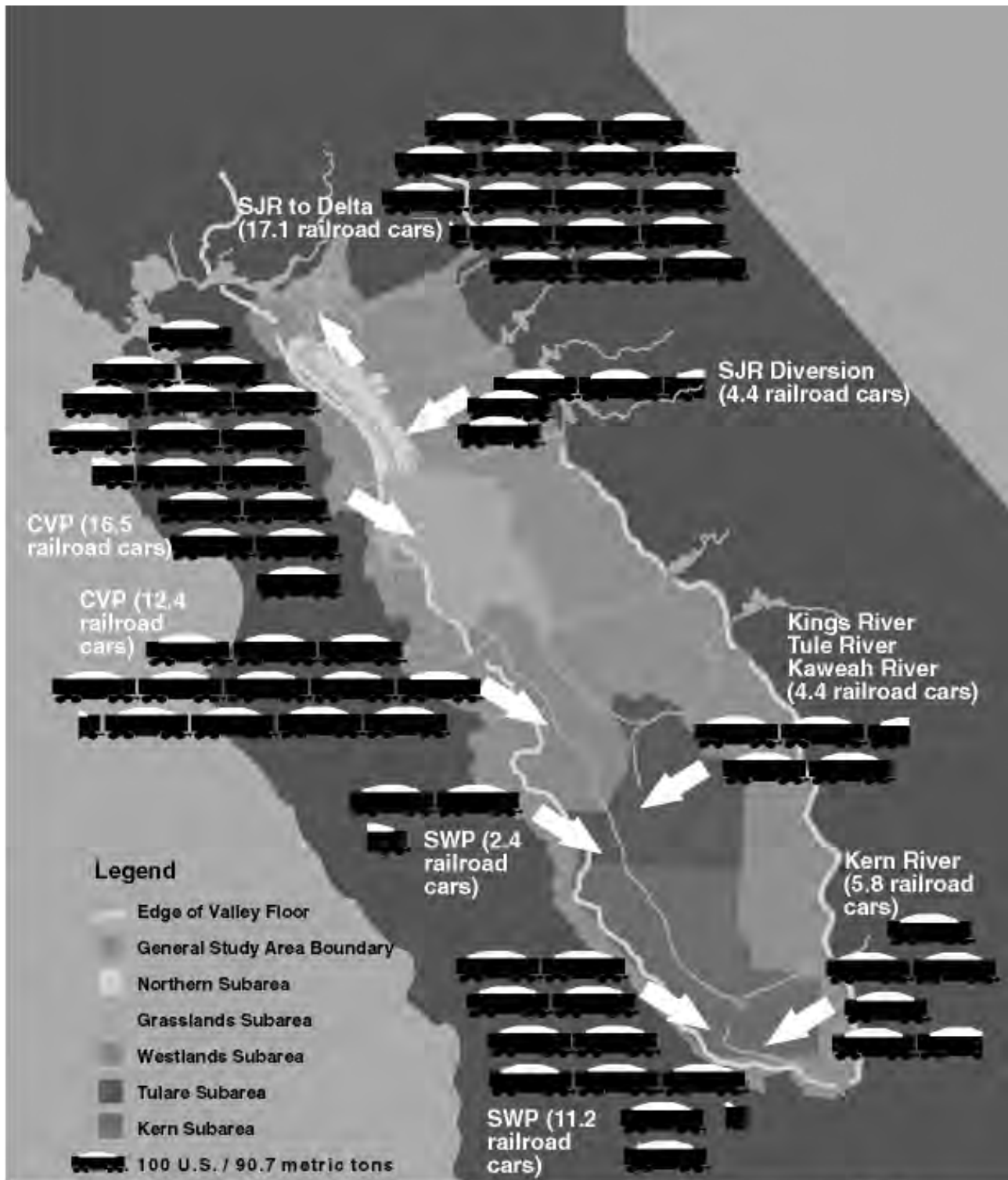
Figure A5. A representation of salt balance in the western San Joaquin Valley showing salt inflow (approximately 40 railroad cars per day) and outflow (approximately 17 railroad cars per day discharged from the Grassland subarea through the San Joaquin River) (printed with permission, Drainage Implementation Program, 1998).
