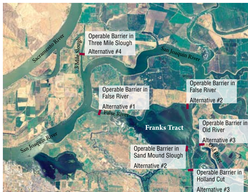
Figure 6.5. Franks Tract Project Alternatives. DWR and USBR propose to implement the Franks Tract Project to improve water quality and fisheries conditions in the Bay-Delta. The project would consist of constructing and operating one or more flow control facilities in the Franks Tract area that would allow better management of hydrodynamic conditions to improve salinity levels and protect at-risk fish species in the Central and South Delta. (Source: California Department of Water Resources 2007, see also http://baydeltaoffice.water.ca.gov/ndelta/frankstract/index.cfm )
