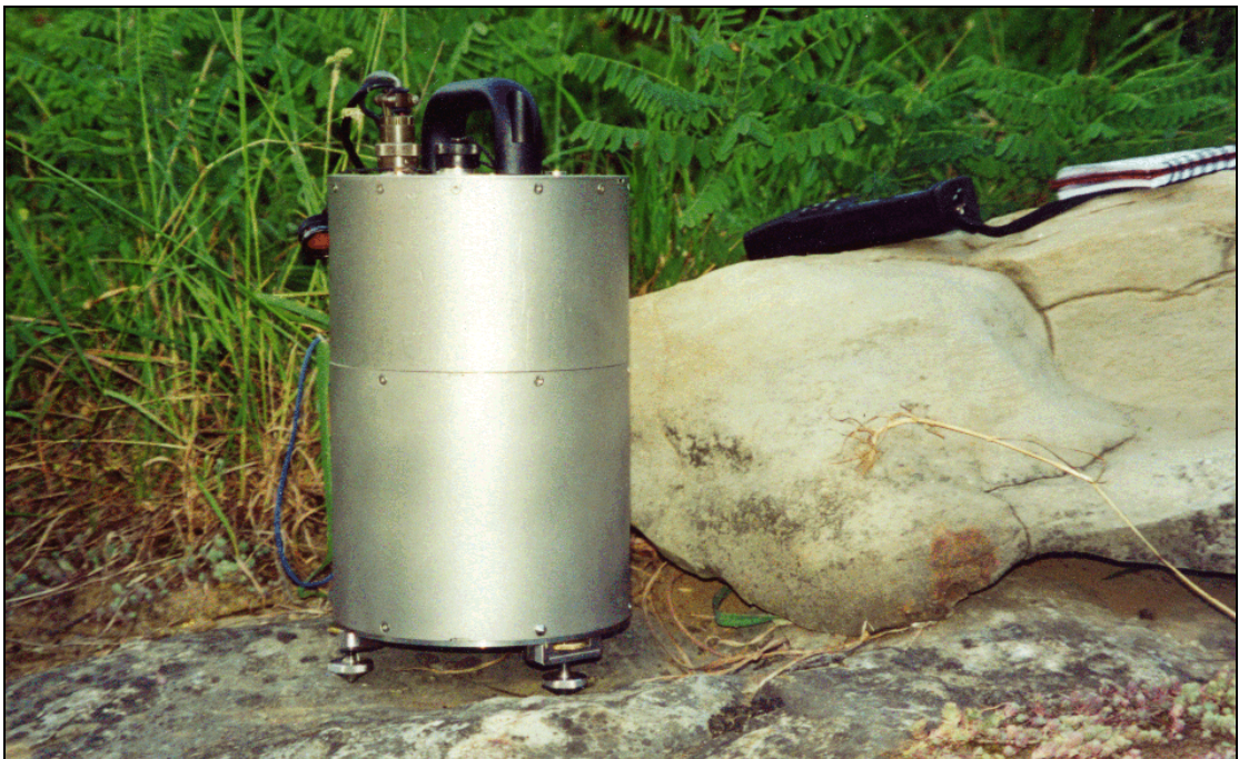
Figure 7.1 Guralp CMG-40TD-1 set up to measure ambient noise at a rock site just outside Düzce, Turkey.
