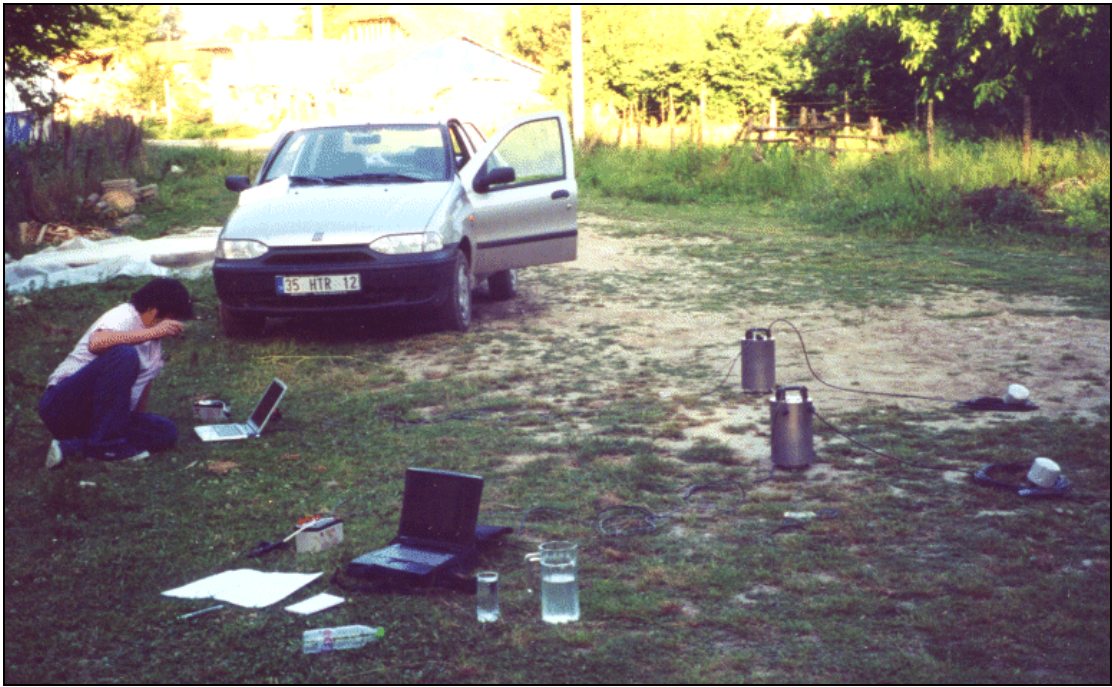
Figure 7.3 Typical field set-up for microtremor measurement. The photograph was taken at location 7.
