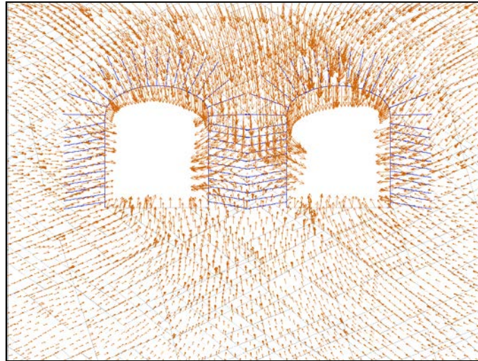
Figure 6-32 Graphical Result of Discrete Finite Element Analysis
