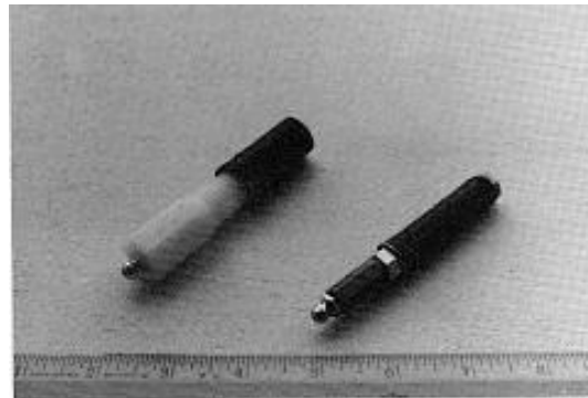
Figure 16-3 Typical Injection Ports for Chemical Grout
