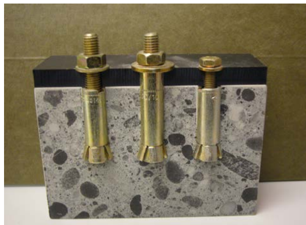
Figure 16-23 Typical Undercut Mechanical Anchors
