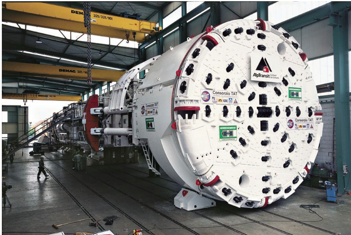
Figure D-3 Herrenknecht S-210 Gripper TBM (Herrenknecht)
