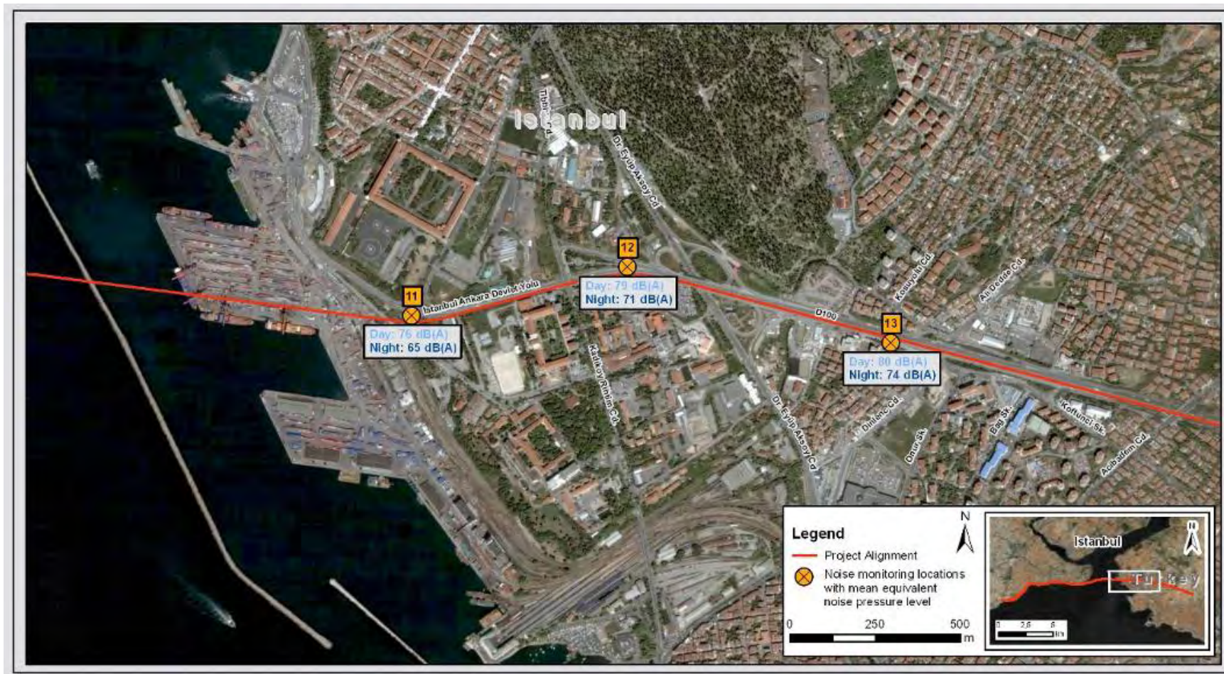
Figure 9-1 Noise Spot-Sampling Locations and Measured Noise Levels for Daytime (L d ) and Night time (L n )
