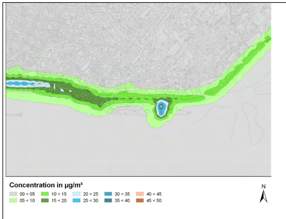
Figure 8-4 Contribution from traffic to annual average NO 2 concentration east of Yenikapi (European side) for the with-Project scenario of 2023
