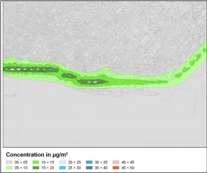
Figure 8-2 Contribution from Traffic to annual average concentration of \text{NO}_2 on Kennedy Cd near Yenikapi in 2009
