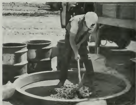
Figure 273. Performing Field Density Test on Zone 3 Material
