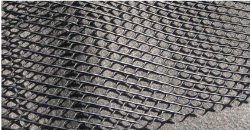
Figure 8.—Geo-net composite – 5-mm biaxial HDPE geo-net, 16 ounces per square yard ( \text{oz}/\text{yd}^2 ) geotextile bottom layer, 6 \text{oz}/\text{yd}^2 geotextile top layer (photo above does not show the top [downstream] geotextile).
