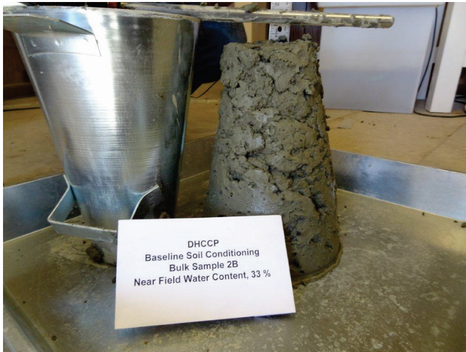
Slump testing of simulated native soil without conditioner.
