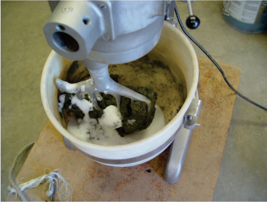
Initial batch of foam conditioner added to simulate RTM.
