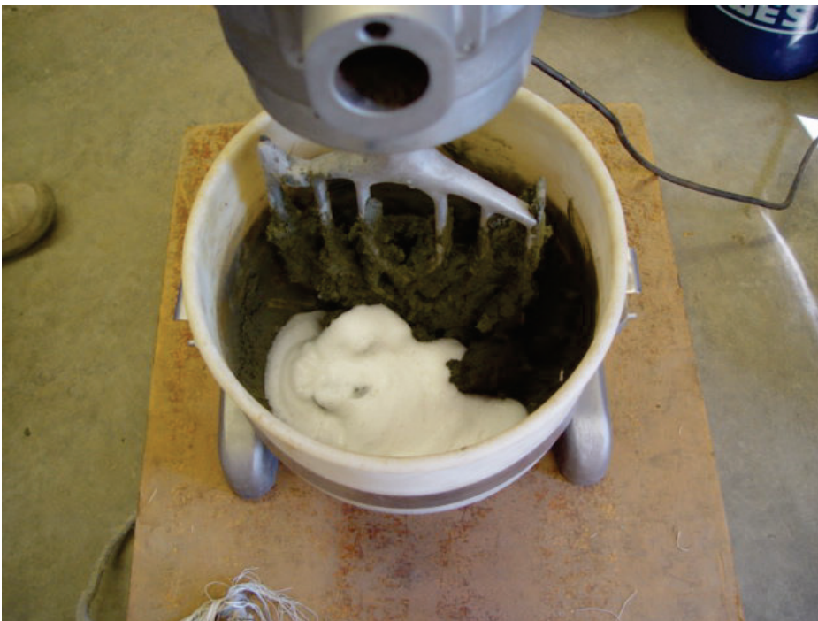
Second (final) batch of foam conditioner added for this testing program.
