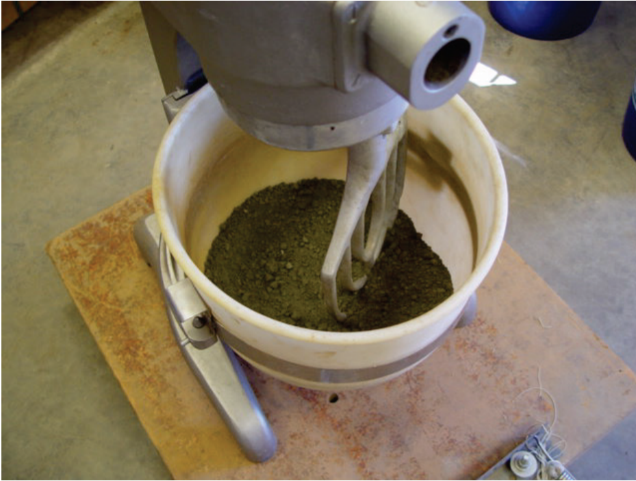
As-received soil moisture content (approximately 17 percent).
