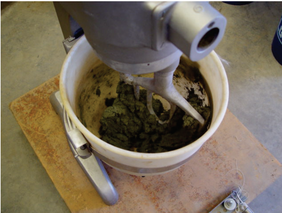
Moisture added to simulate native conditions (approximately 33 percent).
