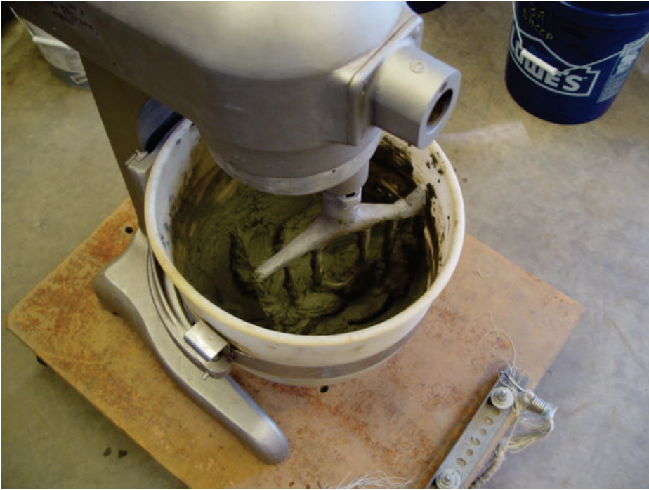
Mixing of soil with second (final) batch of foam conditioner added.
