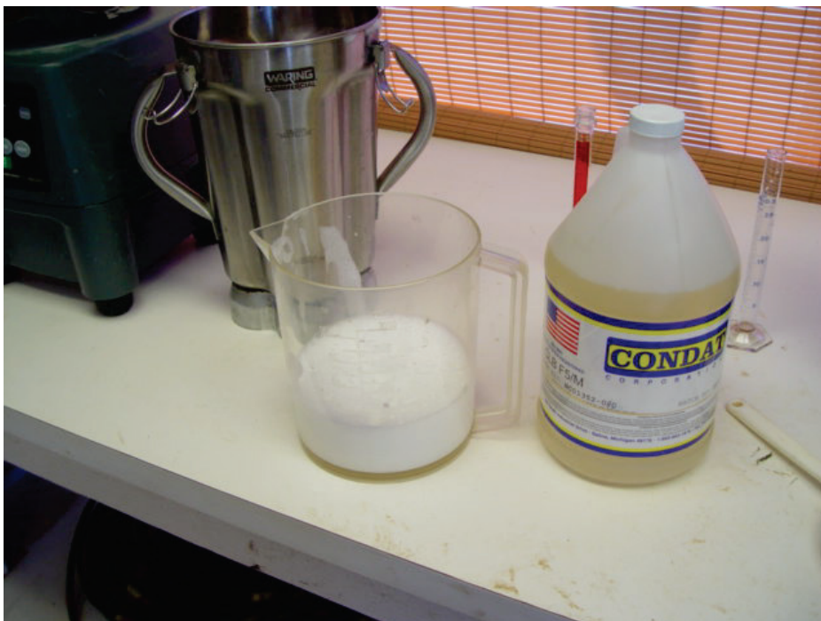
Foam generated from conditioner product using laboratory stirrer.
