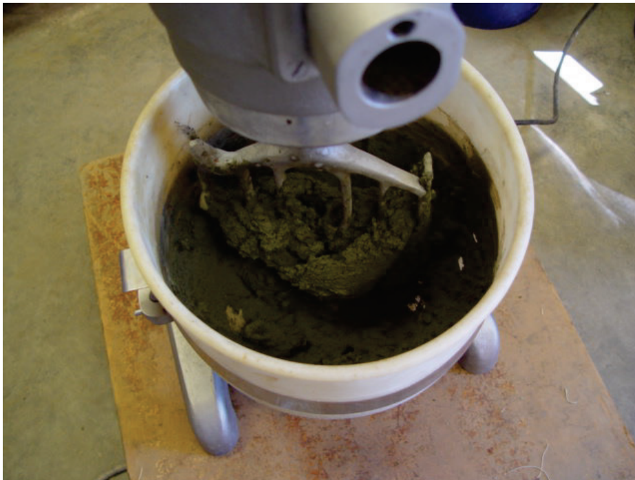
Mixing of soil with initial batch of foam conditioner added.
