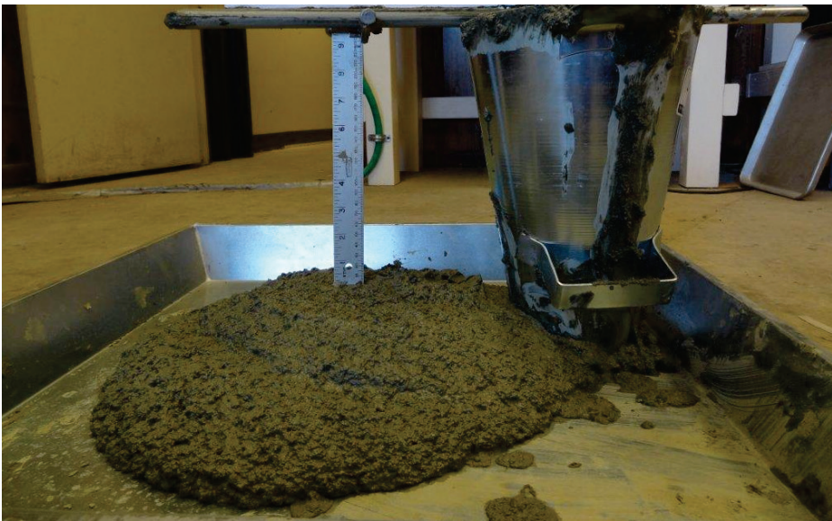
Slump testing of second (final) batch of conditioned soil.
