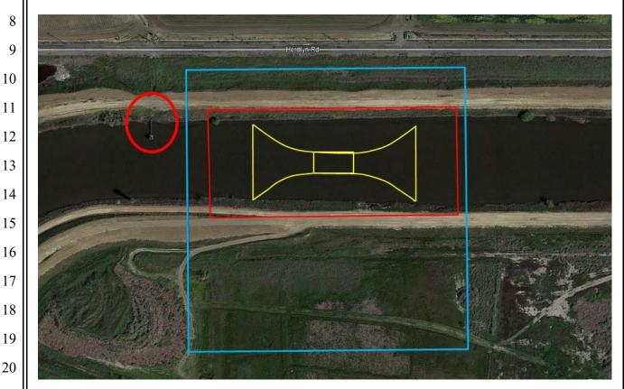
Review of an aerial photograph clearly shows CCLP's intake structure (circled in red), which is located adjacent to, but not within, both the temporary construction footprint (blue box), and the permanent control structure footprint (red box), with the control structure itself shown in yellow outlines. Based on the conceptual engineering completed, the clearance between the CCLP's diversion and the temporary construction footprint is more than 100 feet.
