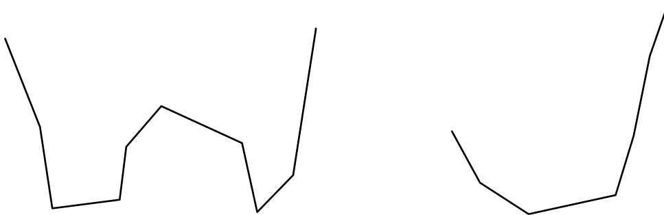
Figure 6-9a: “W” shaped cross-sections are acceptable
