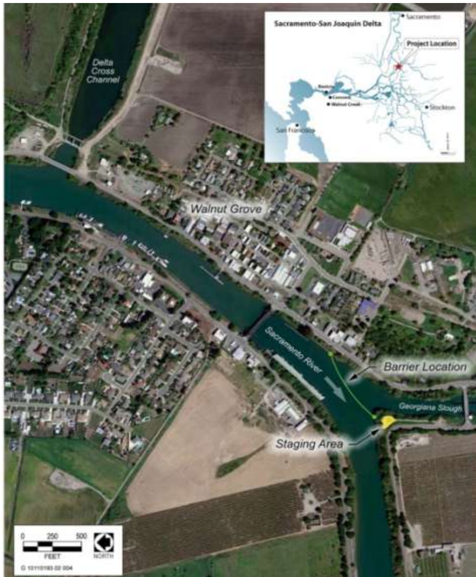
Figure 7-17. Sacramento River in the vicinity of Walnut Grove showing the location of the non-physical barrier tested in 2011 and 2012 (DWR 2012).
