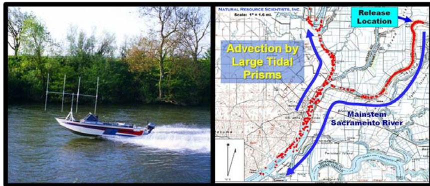
Figure 61. Left picture, mobile telemetry conducted in the north Delta. Photo by Dave Vogel. Figure 62. Right picture, telemetered locations of approximately 100 radio-tagged salmon smolts released in the lower Sacramento River near Ryde (data from Vogel 2001 and Vogel 2004).
