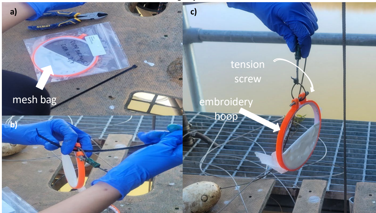
Figure 2. a) outgoing SPATT, b) attach outgoing SPATT to steel cable, c) outgoing SPATT ready for deployment.
