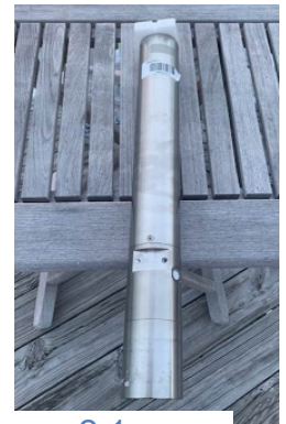
Figure 2.1 Seabird 37 SMP CT Sensor 1
