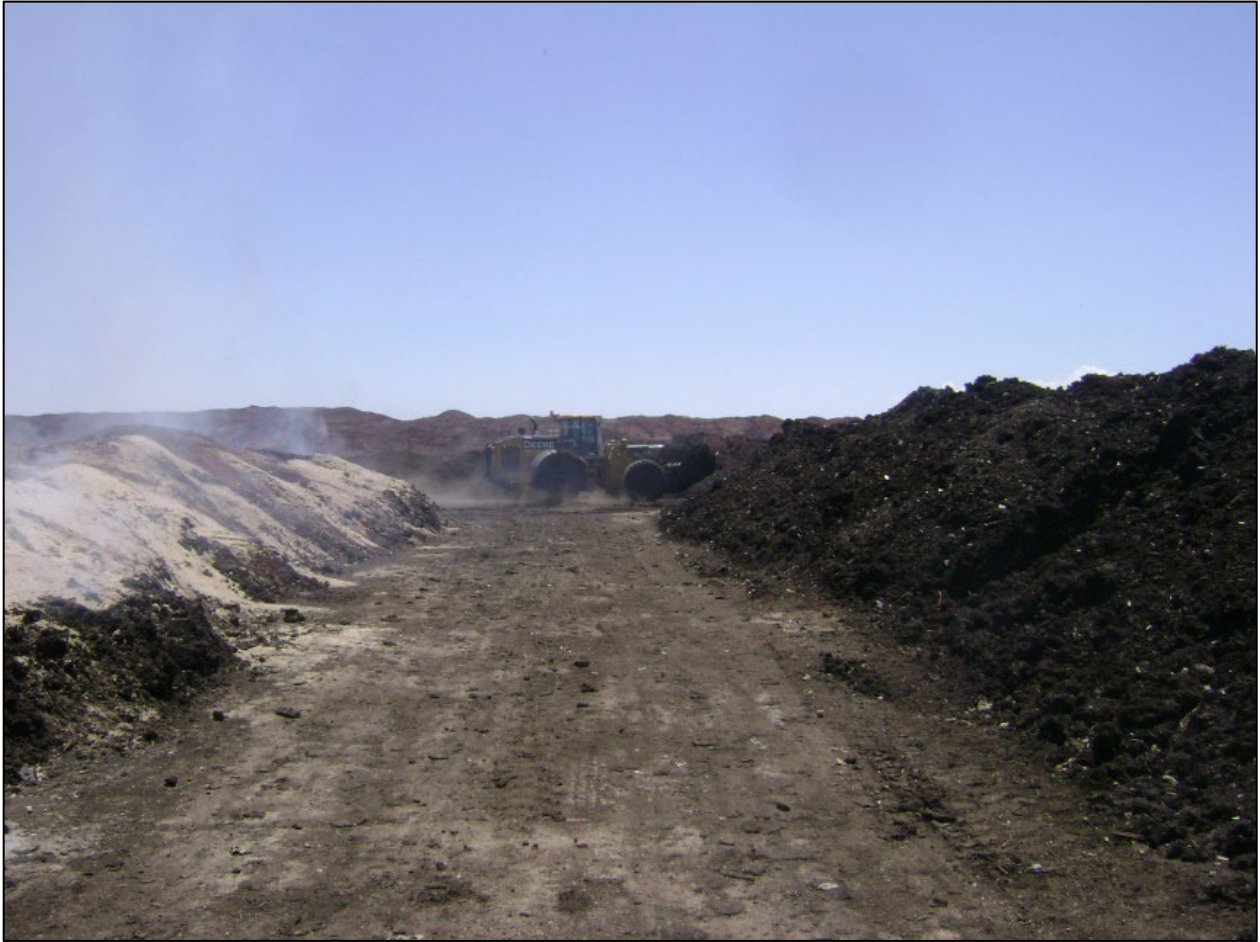
Figure 8.5 - Photo location no. 3, view of interior of site between windrows. The access road between windrows is about 15 feet wide. During the inspection, San Bernardino County Fire indicated that roads need to be a minimum of 26 feet wide between windrows.
