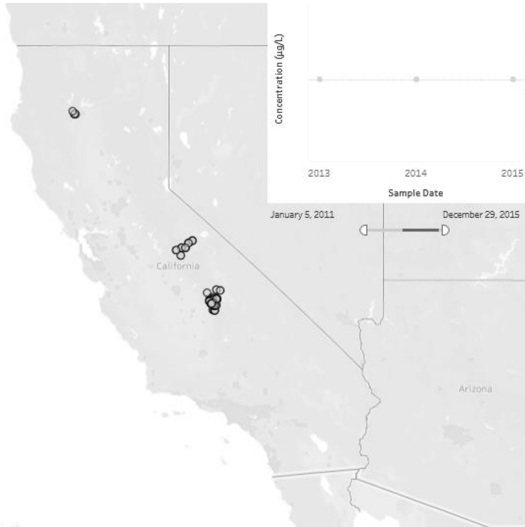
Figure 6.16. Acetaminophen in freshwater, 2011-2015. Teal symbols are detected measurements, grey symbols are non-detect measurements. Concentrations over time in inset plot are in micrograms per liter (ug/L).
