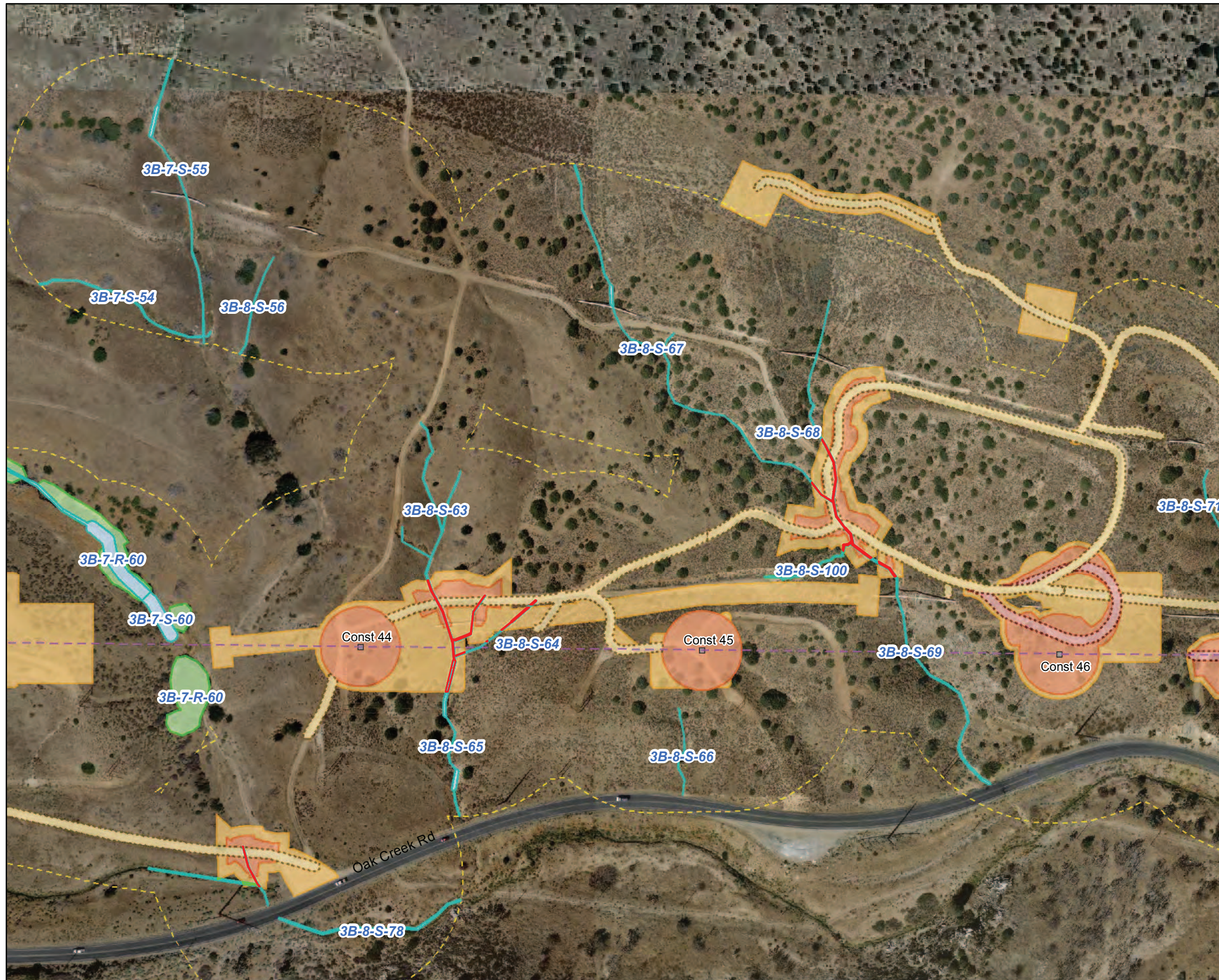
Figure 10 Representative Map of Impacts to Waters under the Water Board and CDFG Jurisdictions (Constructs 44-46 – widening of existing access road, AC Mitigation – zinc ribbon installation, maintenance grading, as well as installation of concrete v-ditch and new concrete outlet, gabion retaining wall, and McCarthy drain) Attachment D Antelope Transmission Project – Segment 3B
