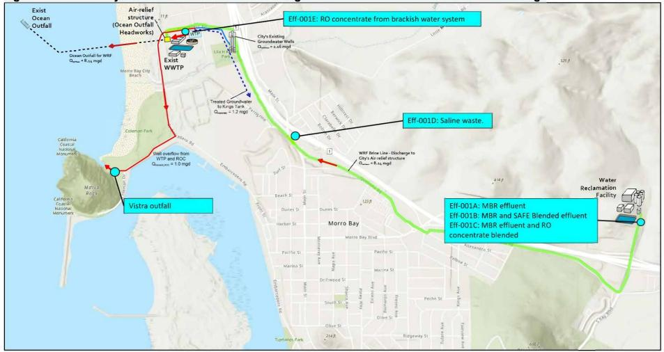
Figure B-3: City of Morro Bay Water Reclamation Facility Site Plan
