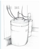
Setting up automated systems to deliver fluids will save employee time and reduce the potential for spills in the shop.
