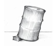
Tipping the drum minimizes liquid from collecting on top of drums.
