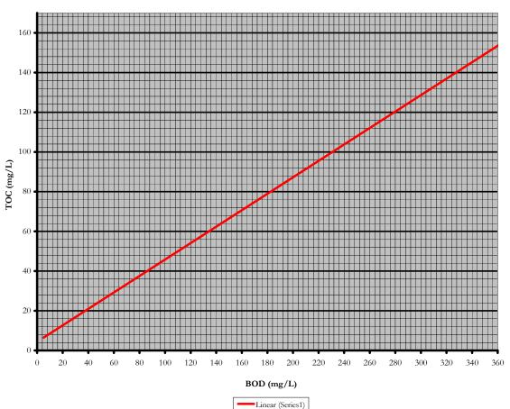
WWTF BOD to TOC chart for Process Monitoring TOC (mg/L) = 0.4141(BOD (mg/L)) + 4.3937 R<sup>2</sup> = 0.9532
