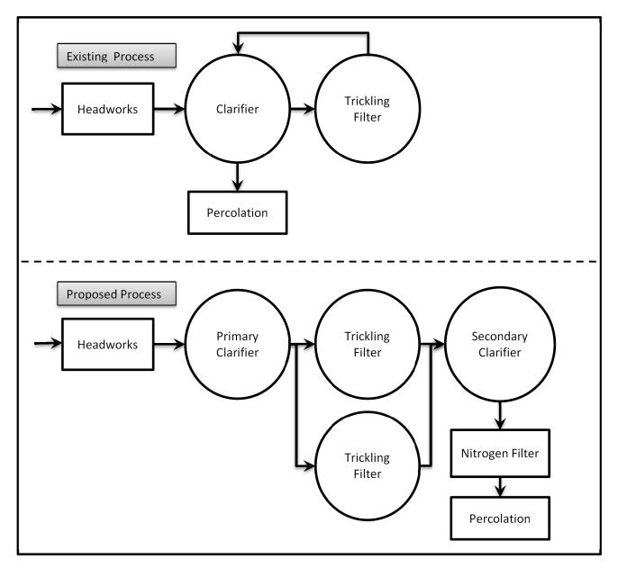
Figure 1 - Existing and Proposed Schematic
