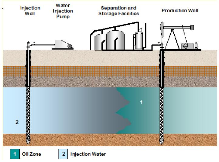
An Example of a Water Flood Injection well; the injected water is being used to push the oil to the production well.
